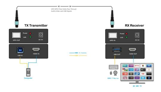
needed, this saves time and cost. Now a fiber optic connection can be made fast and reliable. Using the MPO connector on each end of the Celerity fiber optic cable, a secure snap-lock connection is made to the UFO-GTW-RED-8K-TX and UFO-GTW-RED-8K-RX.
